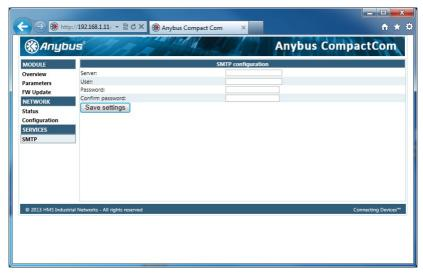
The module needs to be reset for the TCP/IP and SMTP settings to take effect. The Ethernet Configuration settings will take effect immediately.
