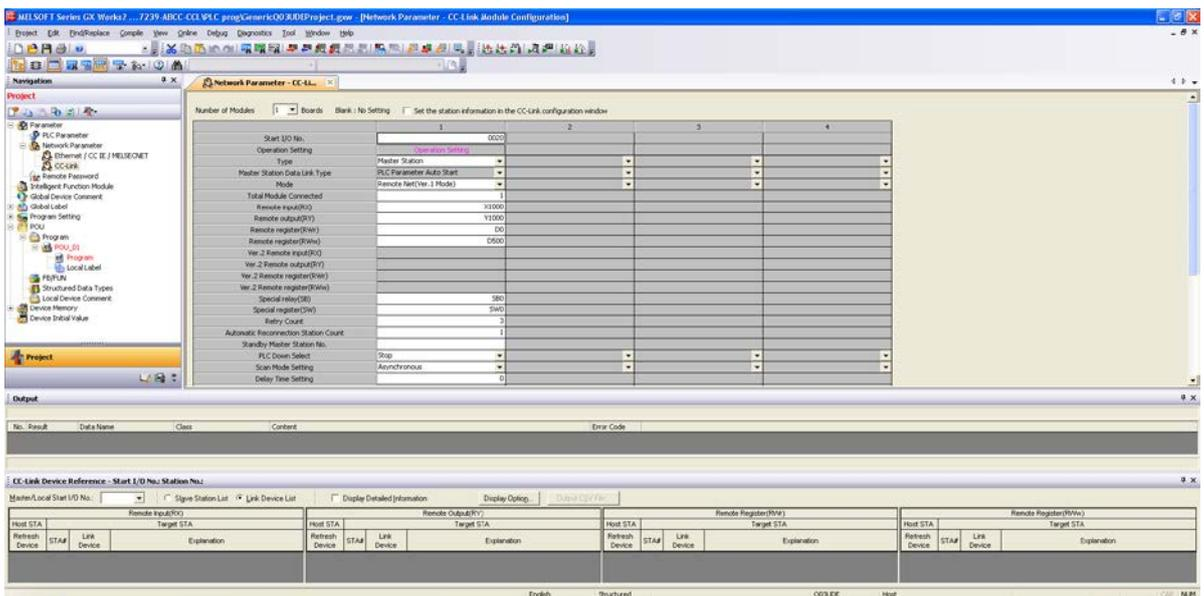
5. Check the check box “Set the station information in the CC-Link configuration window”, to enable the additional configuration window.
