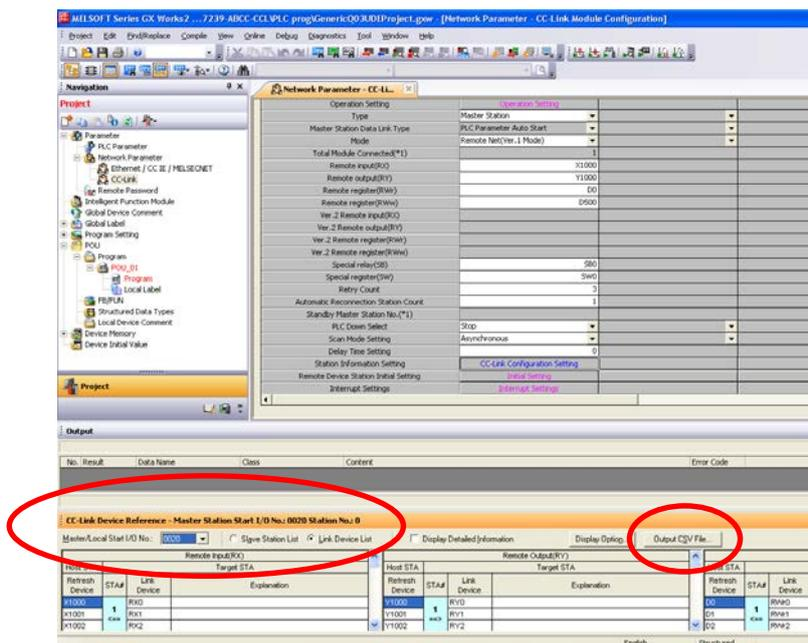
21. In the 'CC-Link Device Reference'-window, press the 'Output CSV File...' button to export the slave mapping into a .csv file (comma separated file). This file can be read into the 'Global Labels' (right click 'Global Label' -> Read from CSV File...).
