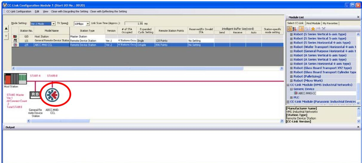
12. If you only have this device you can mark the preconfigured device General Remote Device Station at Number #1 and delete it. Now, only the ABCC-40-CCL is visible.
