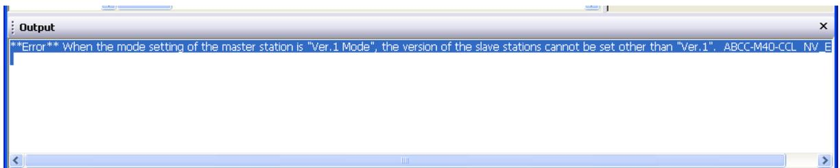
16. Make configuration corrections. In this particular case, slave station “Ver2” is not allowed and is replaced by “Ver1”.
