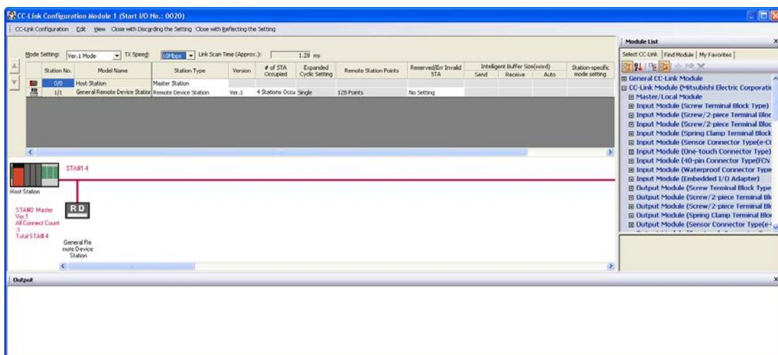
9. Looking under Module List, if we scroll down, we can see the CC-Link module (HMS Industrial Networks AB)->Generic Device”
