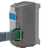
Anybus slot and 50-pin CompactFlash connector on the PCB of the host device
