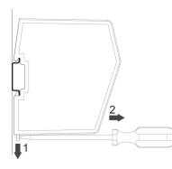
To unmount the module, use a screwdriver to push the DIN-rail fastening mechanism on the back of the module down until it locks in a fixed and open position (1). Then unhook the module from the DIN-rail (2).
