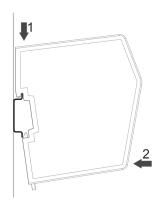
Ensure that the DIN-rail fastening mechanism on the back of the module is in a fixed and closed position, i. e. that it is pushed all the way up.
