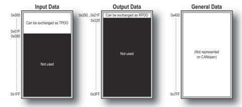
In the Local Object Dictionary input data bytes are mapped to objects starting from index 2000h and output data bytes are mapped to objects starting from index 2100h.
