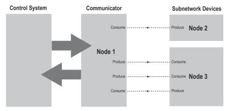
In the figure above, the Communicator 'consumes' data that is 'produced' by a node on the subnetwork. This 'consumed' data can then be accessed from the higher level network. This also works the other way around; the data received from the higher level network is used to 'produce' a message on the subnetwork to be 'consumed' by a node.
