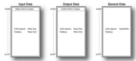
Note 1: The picture shows the maximum available data areas in the Communicator. Not all fieldbuses can access all addresses in the input and output data areas, please see section Data Exchange Model in chapter 1.
