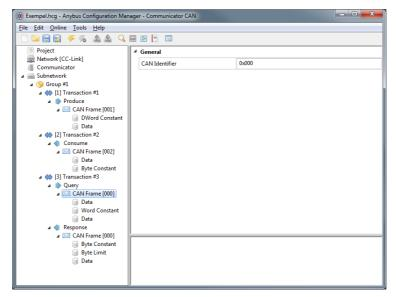
**Note:** A CAN frame can not contain more than 8 bytes of data. It is possible to configure the data area in each frame, but the size of the combination of objects must not exceed 8 bytes.
