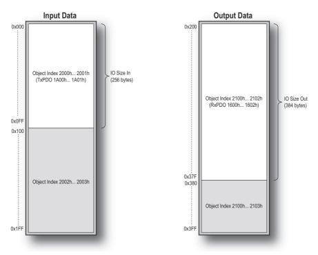
Please note that the two first bytes of the Output and Input Data areas are occupied by the Control/Status Word if this is enabled. Live List and Transmit and Receive Counters are by default mapped to the input memory area from the start address or after the Status Word.
