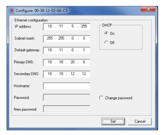
Note that if 'TCP/IP Settings' has been enabled in the Anybus Configuration Manager, any settings received via HICP will be lost in the event of a power loss or reset.
