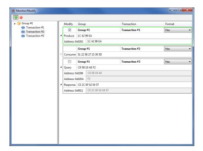
If Modify is enabled, it is possible to change the data values during runtime in Produce transactions and in the Query part of Query/Response transactions, i.e. only the out area of the Communicator can be modified. This will inhibit any data from the industrial network (EtherNet/IP), but input data from the CAN network will still be updated.
