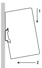
To snap the gateway on, first press it downwards (1) to compress the spring in the DIN-rail mechanism, then push it against the DIN-rail as to make it snap on (2).
