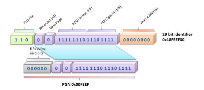
As you can see the PGN 0x00FEEF for this parameter is padded with six leading logic 0 bits, followed by a logic 0 reserve bit, the logic 0 data page bit, and the PDU format/PDU specific fields. Thus the PGN is embedded inside the 29 bit ID between the message priority and the source address.
