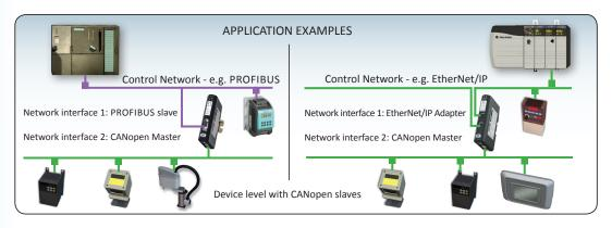
The Anybus X-gateway CANopen family act as intelligent links between two industrial networks. X-gateway CANopen combines simplicity and usability with industrial robustness, making communication across different industrial network types easy and reliable. The X-gateways are easily integrated into any kind of industrial automation system, ensuring a seamless information flow between CANopen and 10 other fieldbus / Ethernet networks.
