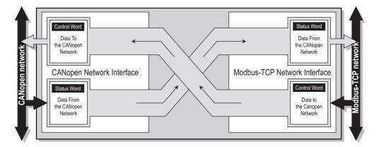
Each buffer holds up to 512 bytes of data, where the first two bytes on the primary network side always are used for control/status information. The remainder 510 bytes gives the theoretical upper limit for the number of data bytes that can be exchanged in each direction. Please note that the actual number of bytes that can be exchanged is highly application and network dependent and can thus be noticably lower than 510 bytes.
