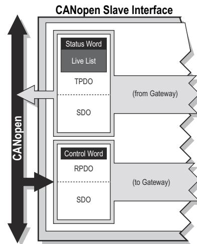
The gateway uses the following PDO mapping scheme by default:
