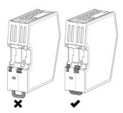
Note: Do not leave the module with the DIN-rail fastening mechanism in a fixed and open position. This may eventually wear the fastening mechanism out so it cannot be used efficiently. Be sure to push the DIN-rail fastening mechanism back into the fixed and closed position after unmounting the module.
