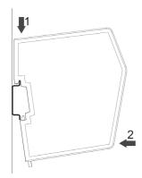
Make sure the DIN-rail fastening mechanism on the back of the module is in a fixed and closed position, i. e. pushed all the way up.
