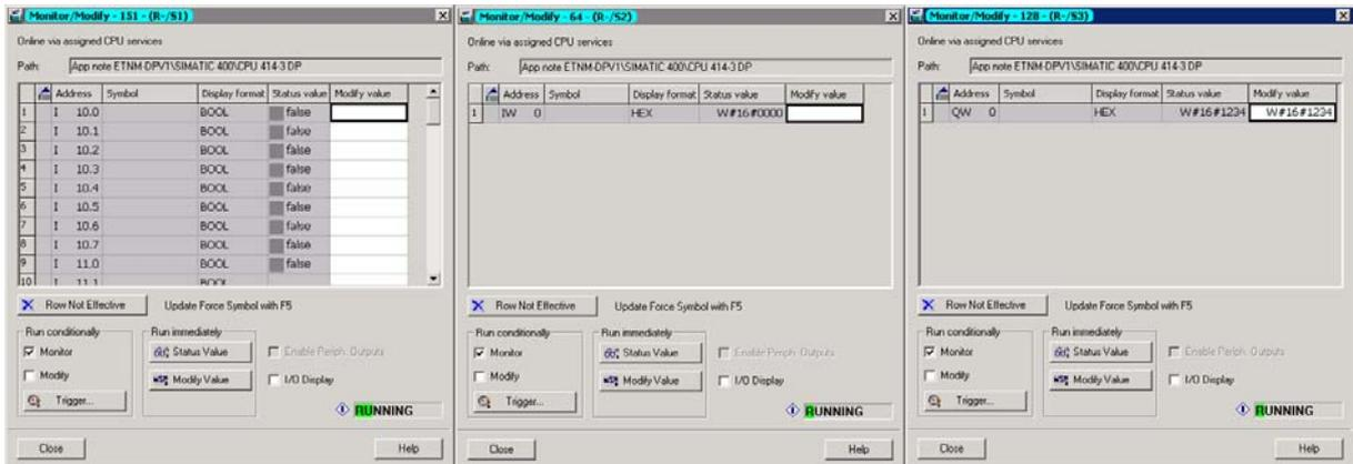
If the Modbus-TCP server is disconnected, the live list will go empty. No transactions will show in the list. The IW0 data will also be empty, since the selection of ‘Clear data to master’ when there is a Modbus-TCP (Network 2) error, on the PROFIBUS DP-V1 configuration page.
