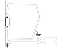
To unmount the module, a screwdriver is needed. Use the screwdriver to push the DIN-rail fastening mechanism on the back of the module down until it locks in a fixed and open position (1). Then unhook the module from the DIN-rail (2).
