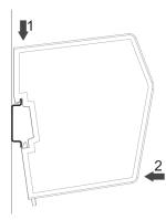
Make sure the DIN-rail fastening mechanism on the back of the module is in a fixed and closed position, i. e. pushed all the way up.
