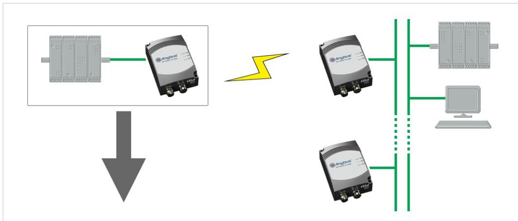
**Fig. 10** Roaming between multiple Wireless Bridges
