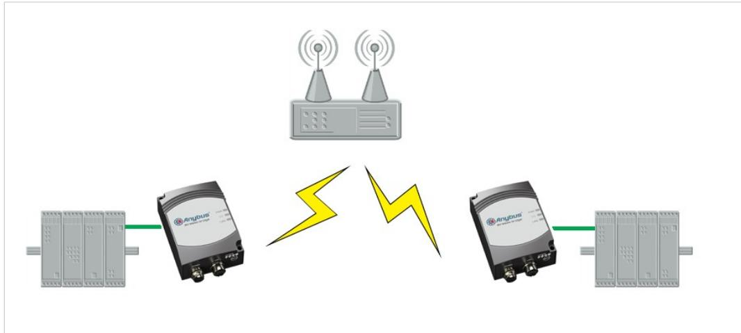
**Fig. 13 Single Clients Connected via WLAN Access Point**
