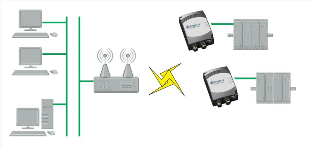
Fig. 16 Single Clients Connected via WLAN to a Wired Network
