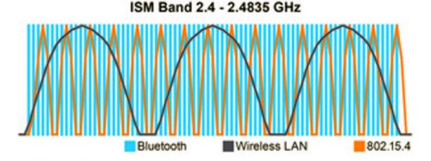
WLAN, Bluetooth and IEEE 802.15.4 work in the same 2.4 GHz frequency band.
