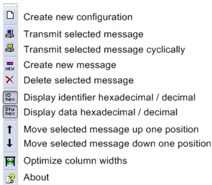
Figure 5.38: Toolbar of the Transmit module
