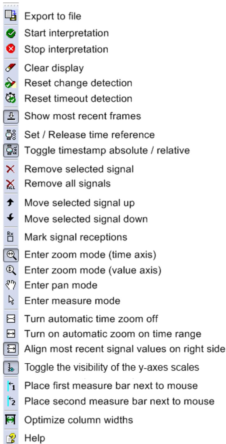
Figure 5.57: Toolbar of the Signal module
