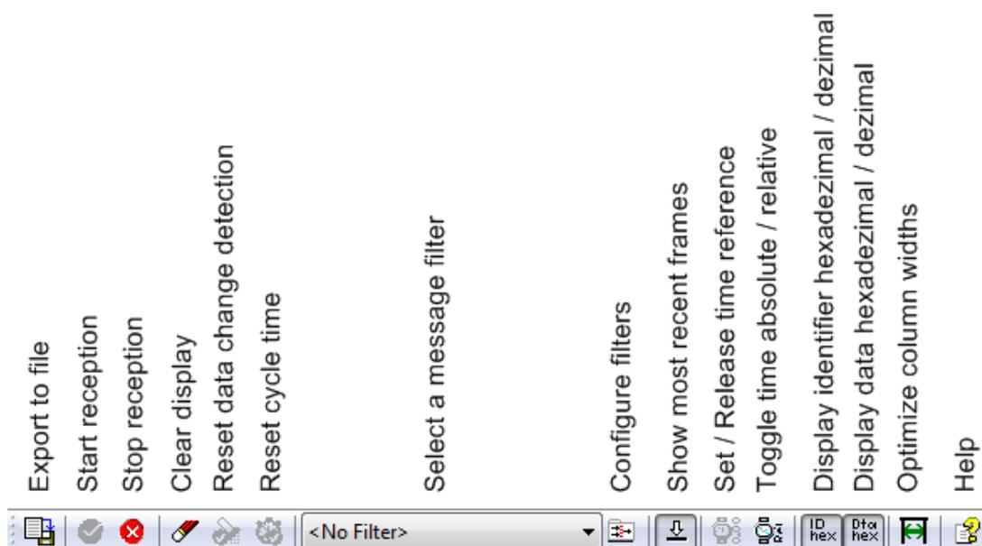
Figure 5.30: Toolbar of the Receive module
