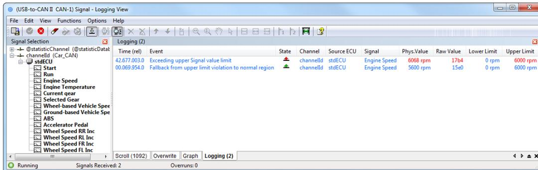
Figure 5.53: Signal module Logging View
