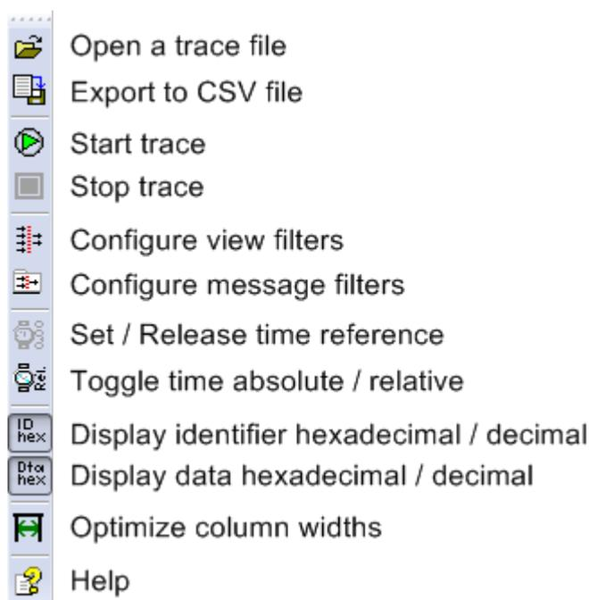
Figure 5.45: Toolbar of the Trace module
