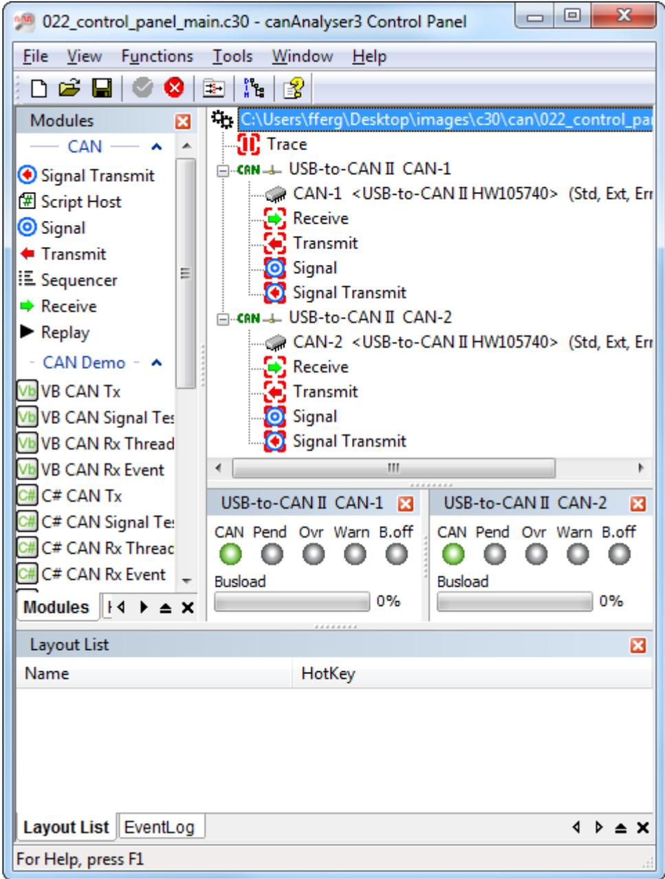
Figure 5.1: The visible fields of the control panel
