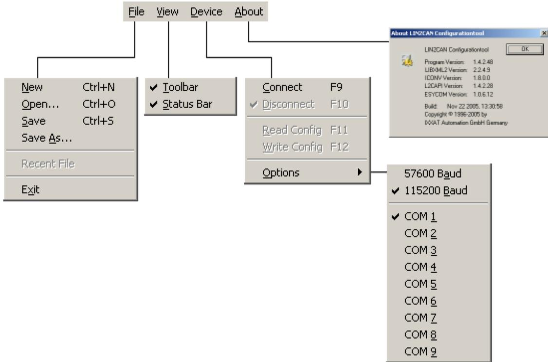
**Fig. 5.9-10: Menu structure Configuration Tool**
