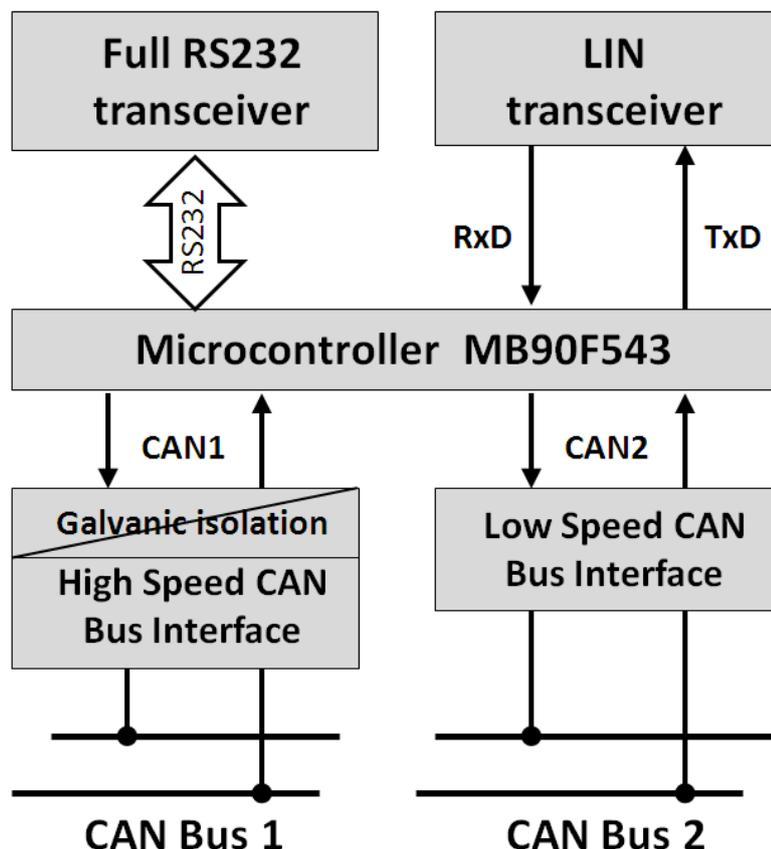
Fig. 2.2-1: Block circuit diagram LIN2CAN Gateway
