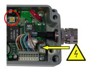
**Notice:** when the product is powered on, please don't touch any elements but the reset button. Take all necessary precautions in order to avoid electric shock and electrostatic discharge.
