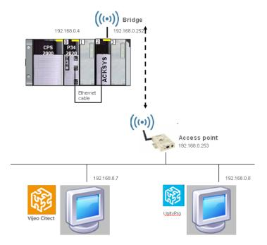
The M340 or M580 CPU, along with the PMXNOW0300, acts as a wireless Modbus-tcp server, whereas VijeoCitect and UnityPro software are Modbus-tcp clients. In that case the Ethernet port of the M340 or M580 CPU is connected to the Acksys PMXNOW0300 wireless module and there is no need for an extra BMX NOE in-chassis module.
