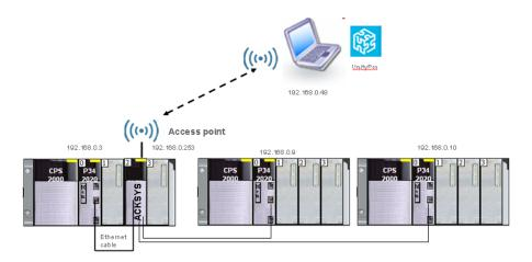
In this network architecture, we take the benefit of the embedded Ethernet switch capabilities of the PMXNOW0300 wireless companion to connect up to 3 M340 or M580 PLCs together. There will be no need for an external Ethernet switch.
