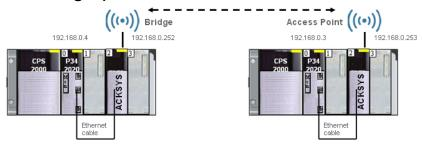
In the use case pictured above we want to read and/or write some of the process data values both ways. We can use the READ\_VAR / WRITE\_VAR function blocks just like if both PLCs were connected on an Ethernet cable. We do not need any extra BMX NOE in chassis module.
