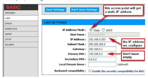
Note: Most of the configuration parameters are already set by default and do not need to be changed; we will just configure a network name (SSID) and select a security mode to encrypt the communication
