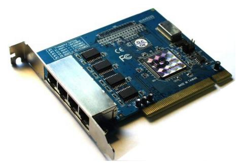
Figure 8: VScom 400H RJ45 PCI
