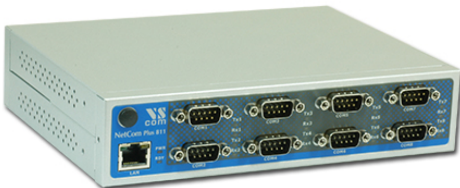
Figure 6: NetCom Plus 811 / 813 Front side
