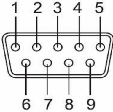
**RS-422 Signal Pin-outs of DB-9 Male (CN2, CN3)**
