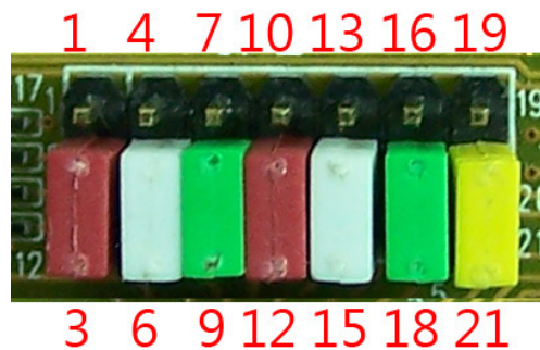
Example jumper block setting ( RS-422 mode )
