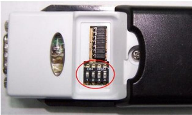
**4-pin DIP switch for operating mode selection**
