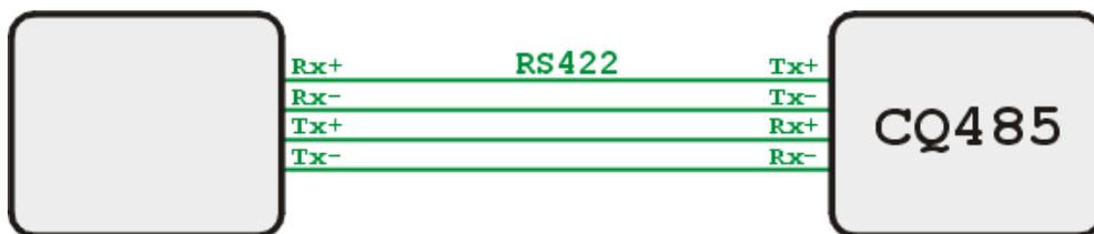
Fig. 10 - An example of a system with an RS422 line interconnection.
