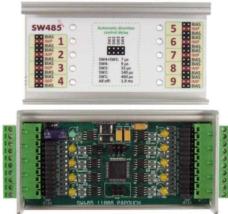
Fig. 4 – electronics board inside the box and information label on the bottom side of the lid
