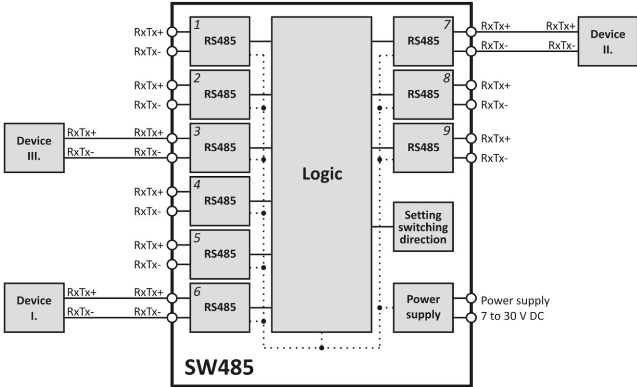
Fig. 1 – block diagram and connection of two devices
