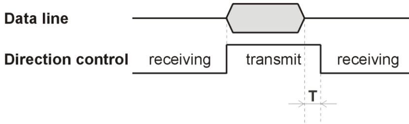
Fig. 3 – switching delay
