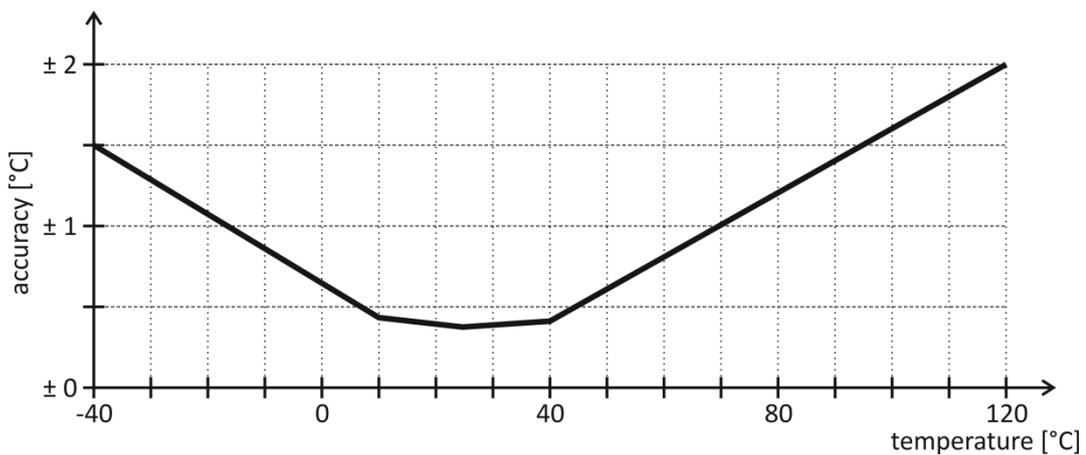
Fig. 11 – temperature measuring accuracy for THT2 sensor
