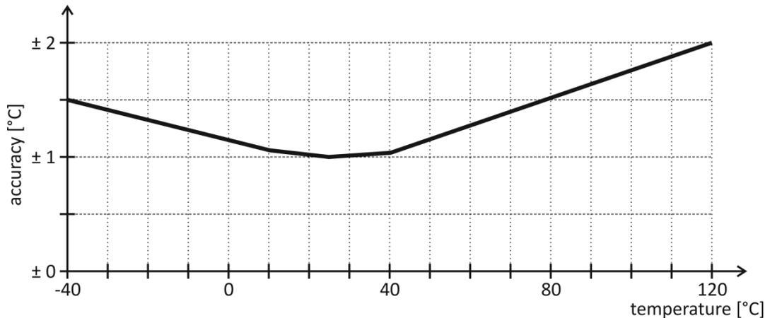
Fig. 12 – temperature measuring accuracy for THT2 I sensor
