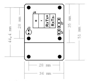
Figure 5 – Board with Electronics Drawing
