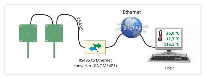
The module measures temperature using an integrated unit with the accuracy of  $\pm$  0,5°C. The TQS3 module contains an indicator which blinks to signalize the ongoing temperature measurement.
