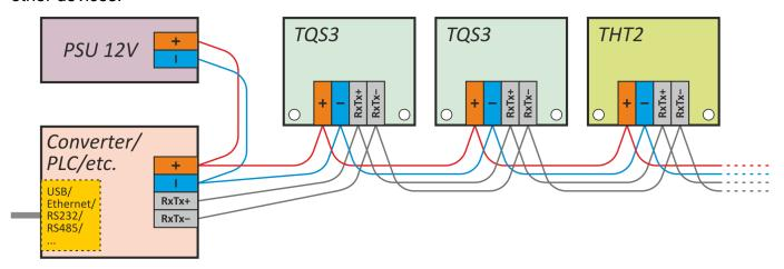
Fig. 2 – example of TQS3 connected to a converter and other devices
