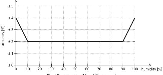
Fig. 10 – accuracy of humidity measuring
