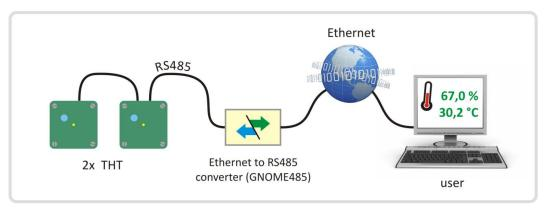
Fig. 1 – Example of THT2 sensors connection to PC (directly or over Ethernet)
