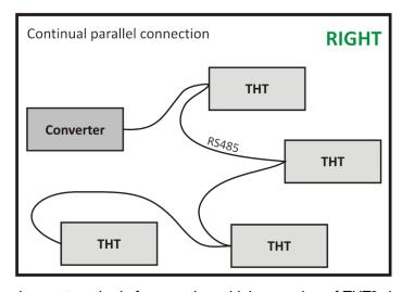
Fig. 6 – Incorrect and correct method of connecting a higher number of THT2 devices via RS485
