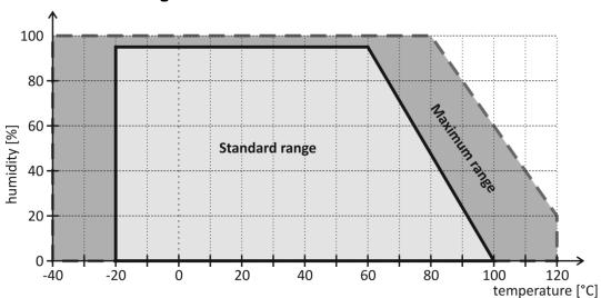
Fig. 13 – working and maximum temperature range
