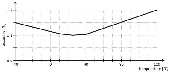
Fig. 12 - temperature measuring accuracy for THT2 I sensor
