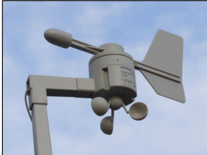
Fig. 2 – wind speed and direction sensor
