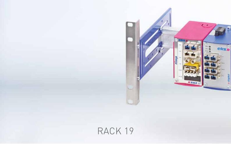
UNIVERSAL 19" DIN RAIL CARRIER Rack 19" can be used for the mounting of a DIN rail in a horizontal or vertical way. Furthermore, it is suitable for wall mount. The DIN rail can be adjusted in depth. There are 3 different angles for 19" mount. They are used for adjusting the height and can be changed even if they are mounted.
