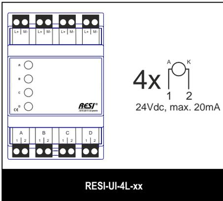
Our signal modules offer four LEDs to show the current status or errors of machines and systems. The modules are suitable in every area of building automation like HVAC, light, electric engineering or security.
