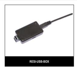
This converter offers an USB1.1/USB2.0 to serial interface to connect to a serial line based on RS232 or RS485 signals via USB. The converter is based on the Silicon Labs CP2103 chipset. In case of a RS485, automatic TX/RX flow control is done by the USB chipset. The module offers an USB socket to connect the USB cable to the host. The serial bus is connected via a removable 3 pin terminal. A switch defines the type of the serial interface: Either RS232 or RS485.
