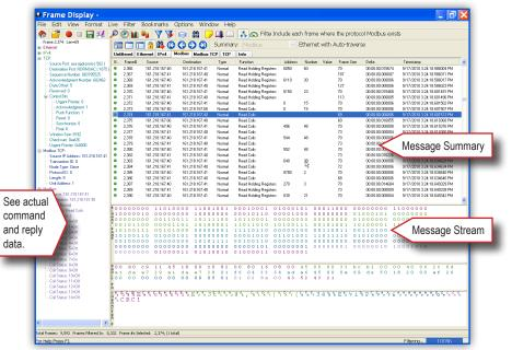
Together with our comprehensive line of USB hardware interfaces, Frontline's NetDecoder protocol analyzer monitors and provides detailed timing, data, and messaging information for a wide range of communications protocols.
