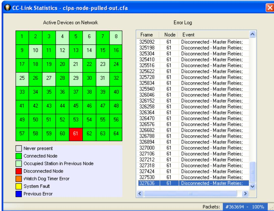
**Figure 21: Node Disconnected and Master Retries**
