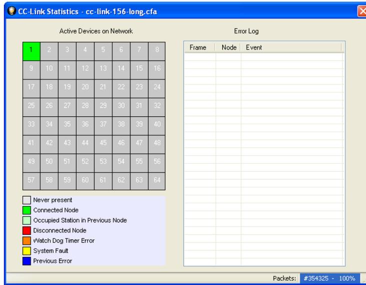
**Figure 18: Network with Only One Node**
