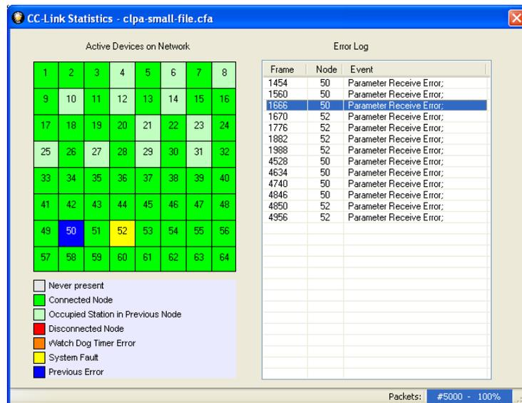
**Figure 19: Grid with Connected Nodes and Occupied Stations**
