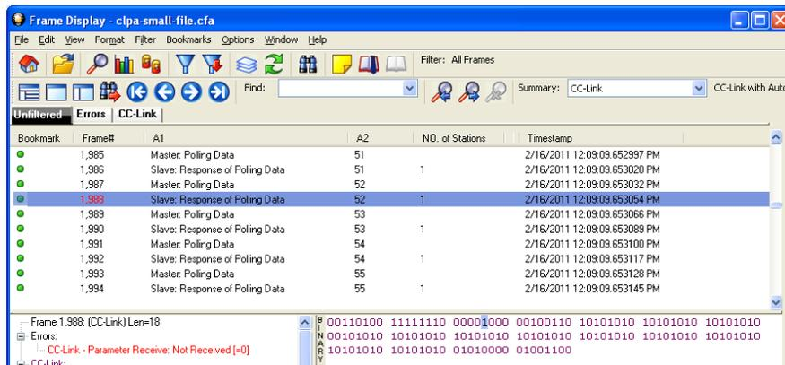
Figure 25: Node 52 with Parameter Receive Error
