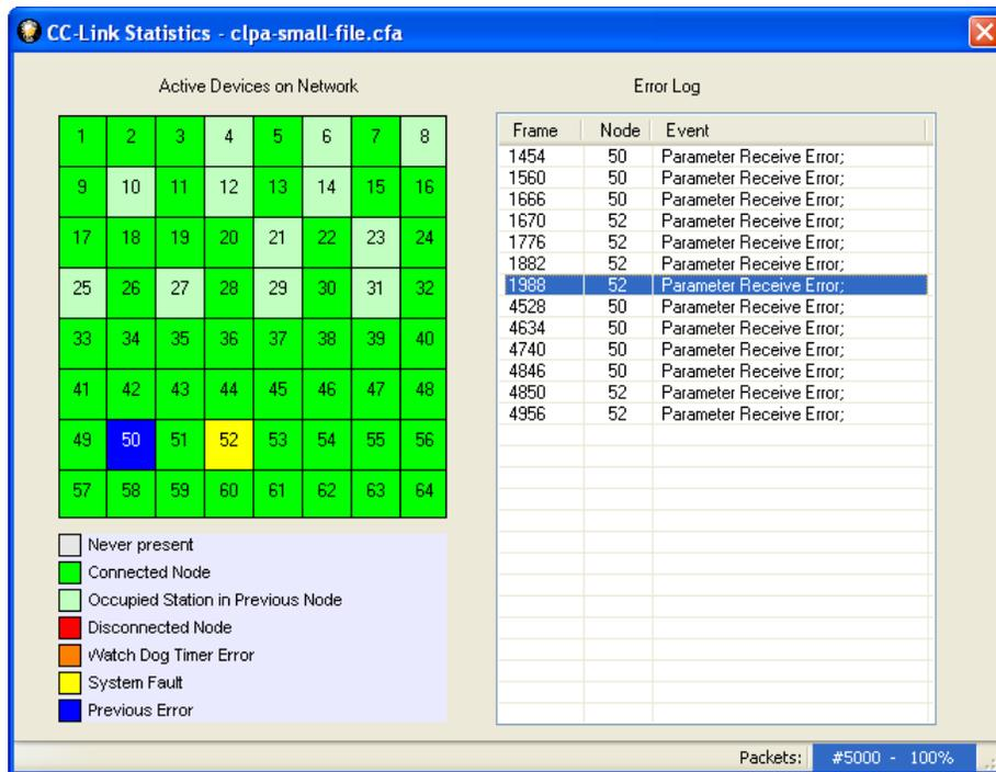
Figure 24: Node 50 and Node 52 with System Fault
