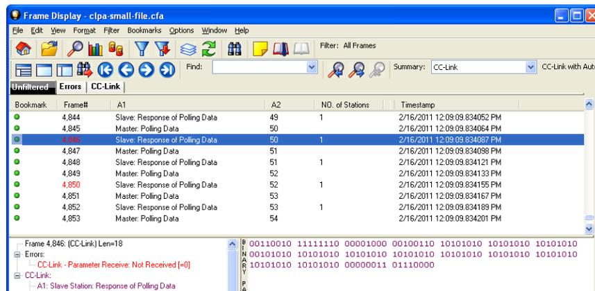
Figure 26: Node 50 with Last parameter Error
