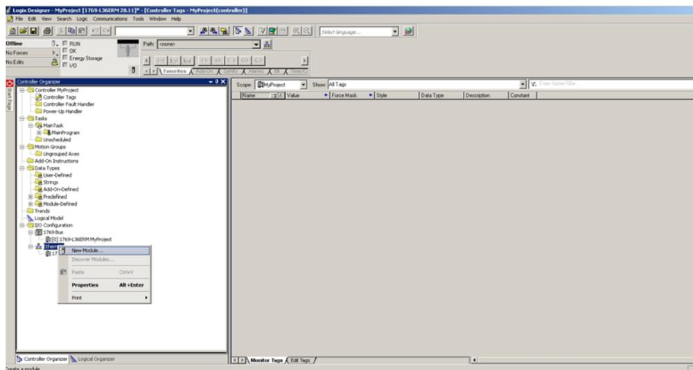
2. Select the HMS-EN2MB-R Linking Device (catalogue number: HMS-EN2MB-R) and click “Create”.
