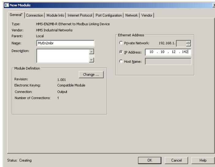
4. In the “Module Definition” window, launch the configuration manager for the HMS-EN2MB-R linking device.
