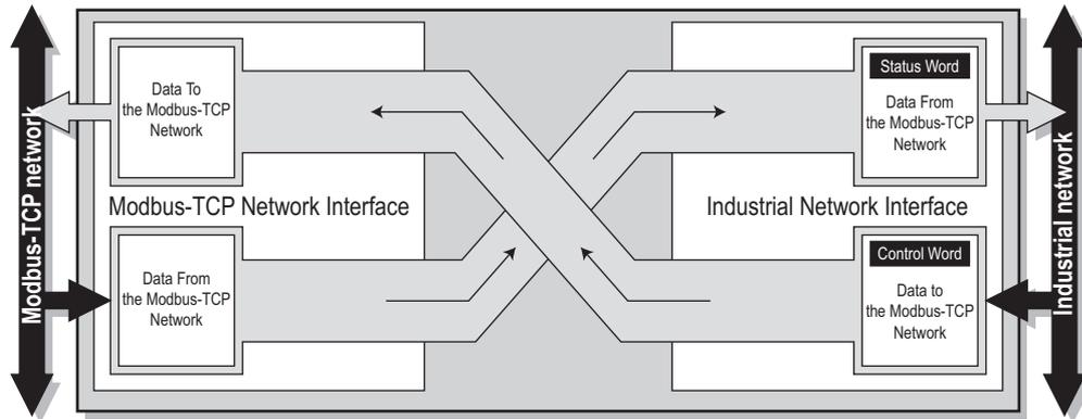
Each buffer holds a maximum of 4096 bytes of data. The first two I/O mapped bytes in either direction can be dedicated for control/status information, and another eight bytes of data coming from the Modbus-TCP network can feature a live list. Please note that the actual number of bytes that can be exchanged is highly network dependent.
