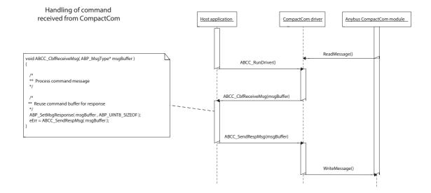
The driver uses non-blocking Anybus CompactCom message handling. This means that a state machine must be used to keep track of commands and responses.
