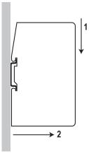
To snap the gateway off, push it downwards (1) and pull it out from the DIN-rail (2), as to make it snap off from the DIN-rail.
