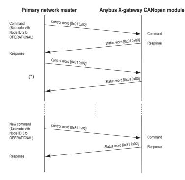
(\*) The communication is performed in an ongoing ping-pong fashion. The same command is sent repeatedly, but as long as the toggle bit is not changed, the module will ignore the message. A new command is signalled by the toggle bit changing value.
