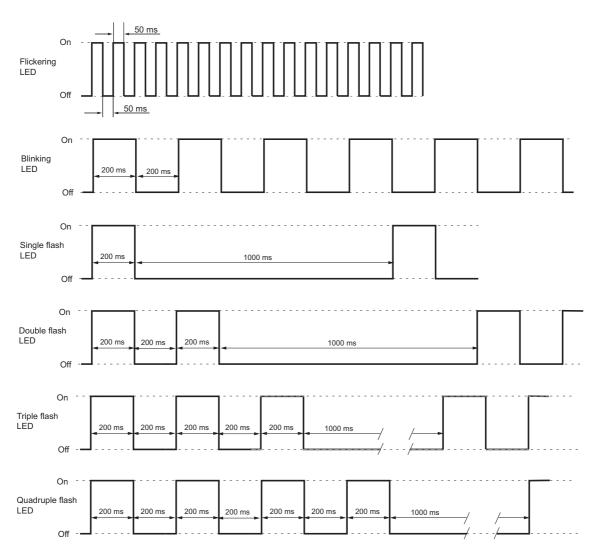
The LEDs on the front of the module change their behavior according to the status of the module. This appendix gives the timing diagrams for the different indications, described in "Status LEDs" on page 7.
