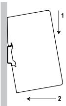
To snap the gateway on, first press it downwards (1) to compress the spring in the DIN-rail mechanism, then push it against the DIN-rail as to make it snap on (2).
