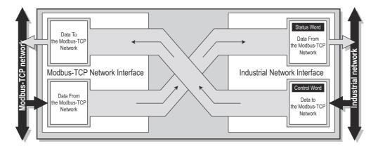
Each buffer holds a maximum of 256 bytes of data. The first two bytes in either direction can be dedicated for control/status information, and another eight bytes of data coming from the Modbus-TCP network can feature a live list. Please note that the actual number of bytes that can be exchanged is highly network dependent.
