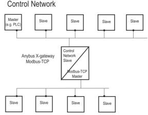
The DeviceNet fieldbus adapter interface is configured with a standard device description Device Level with Modbus-TCP Slaves file (GSD/EDS) and the standard engineering tool of the PLC. No programming is required.
