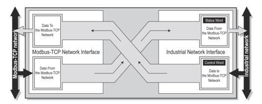
Each buffer holds a maximum of 256 bytes of data. The first two bytes in either direction can be dedicated for control/status information, and another eight bytes of data retrievable from the X-gateway by the PROFINET network can feature a live list. Please note that the actual number of bytes that can be exchanged is highly network dependent.
