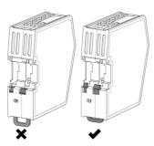
Note: Do not leave the module with the DIN-rail fastening mechanism in a fixed and open position. This may eventually wear the fastening mechanism out so it cannot be used efficiently. Be sure to push the DIN-rail fastening mechanism back into the fixed and closed position after unmounting the module.
