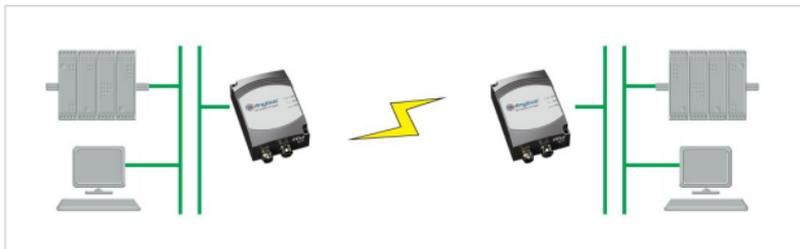
This example describes two Wireless Bridges in PANU mode connecting two Ethernet network segments.
