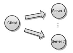
At Low Energy level, the Client-Central is scanning for the Server-Peripheral. When the Server-Peripheral starts advertising the Client-Central finds the Server-Peripheral and initiates the connection.
