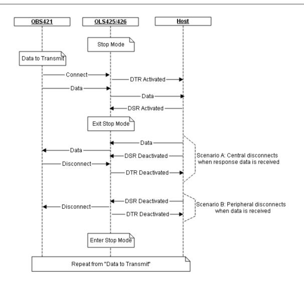
There are two ways to terminate the connection. In scenario A, the host of the peripheral must send a response and when received by the central, it disconnects. Another option, scenario B, is for the host of the peripheral to disconnect once the expected data is received.
