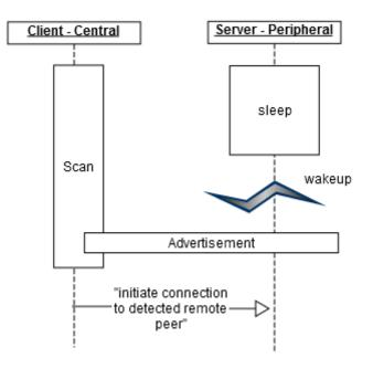
The connection attempt can (for some modules) be initiated with the connect (AT\*ADCP) AT command.
