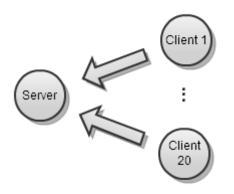
The Client-Peripheral then makes a directed advertisement which is targeted to a specific Server-Central. If that specific Server-Central detects the advertisement, it will initiate a connection. Hence, it is still the central that initiate connections but at a Serial Port Adapter concept level, the peripheral will be configured as the client and the central as the server.
