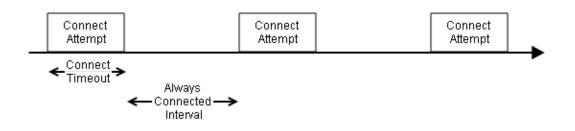
By default, the connect timeout is 5 seconds and the always connected interval is 10 seconds. The connect timeout and the always connected interval can be configured using the ATS6007 and ATS6010 S-register AT commands. Please note that for Bluetooth Low Energy, the module will not do a scan between the connect attempts. Scanning is only performed during a connect attempt.
