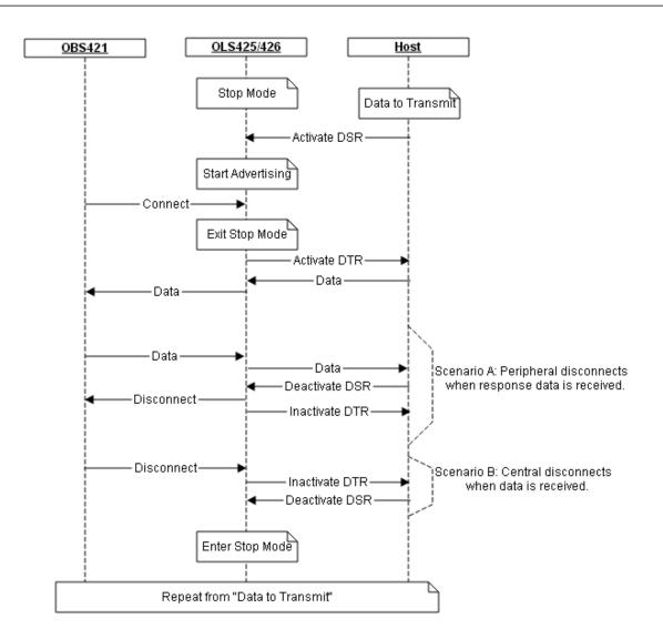
There are two ways to terminate the connection. In scenario A, the central must send a response and when received by the host of the peripheral, it disconnects by deactivating DSR. Another option, scenario B, is for the central to disconnect once the expected data is received.
