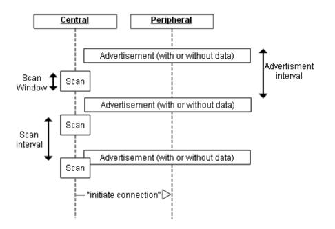
One important advertisement parameter is the advertis*ement interval*. A short interval will allow for faster detection and connections but it also means that the power consumption increases for the peripheral during the advertisement.
