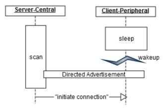
The client module is configured to automatically "setup the connection". The default client profile (AT\*ADDCP), the write remote peer (AT\*ADWDRP) and the number of remote peers (AT\*ADNRP) AT commands must be used for the Client-Peripheral. The remote peer is the server that the client is configured to setup a connection to.
