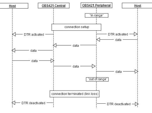
The OBS421 DTR pin is configured to show the connection status. Hence, it can be used like a traditional CD (Carrier Detect).
