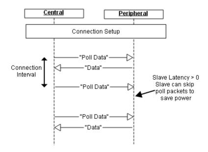
It may be necessary to configure both advertisement and connection intervals to optimize for a specific use case. This may mean compromising between fast connection and response times and low power consumption.
