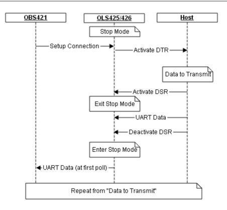
The OLS425/426 is configured as a server-peripheral and the OBS421 as a client-central. For basic connection setup, see section <u>Basic Connection Setup Configuration</u>
