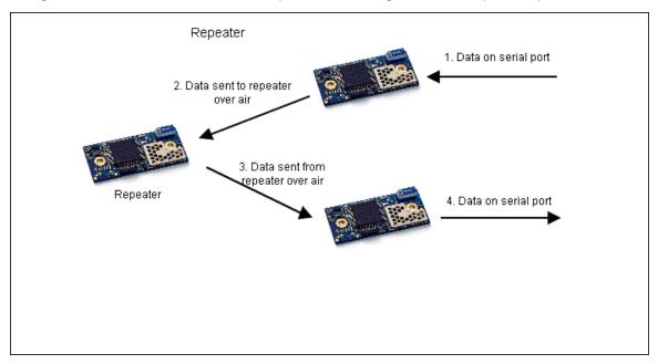
The *auto forward* parameter enables the repeater functionality. Of course this is only useful for the multipoint case since it requires at least two parallel Bluetooth connections. If enabled, data received from one Bluetooth channel is transmitted to all other Bluetooth channels. Data transmission over the serial port is disabled and it can only be used to enter the *AT Mode* and then execute AT commands.
