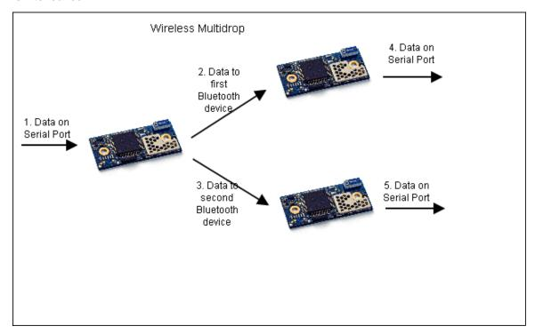
In Extended Data Mode it is possible to transmit data to a specific remote device and to know from which remote device data is received.
