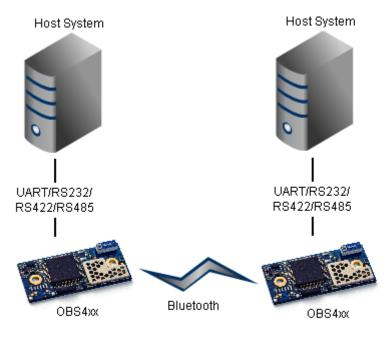
The basic functionality is to transfer data between the serial port and a Bluetooth link. It is possible to configure a module to automatically setup a connection and/or accept an incoming connection. Configuration is done using AT commands.
