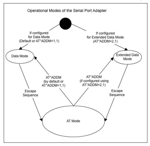
In *AT Mode* the module is configured using AT commands. For details on available AT commands see [1]. Please note that the module does not accept incoming connections in AT mode. It is, however, possible to set up an outgoing connection using the AT\*ADCP command.
