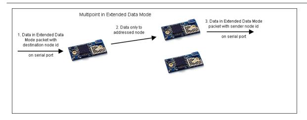
For the multipoint case it is important to consider the master/slave role (which is not the same as client/server). If a device has multiple Bluetooth connections active and if the device is master for all the connections, this is a piconet. If the device is master for all of the connections expect one where it is the slave this is called a scatternet. Performance for a piconet is better and more robust than for a scatternet. Also, for a scatternet only 6 parallel channels can be achieved.
