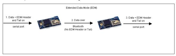
Note that, over air, there is no *Extended Data Mode* protocol data. Over air only "raw" data is transmitted in the same way as for *Data Mode*. Hence, it is possible for one side to be configured for *Extended Data Mode* and the other side standard *Data Mode*.
