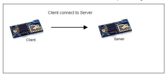
The client and server role is often mistaken for master and slave role. The master/slave role is defined at a lower level (master polls slave at radio level) and has nothing to do with client and server. By default the client will become master and the server will become slave. However, a master/slave switch during or after connection set-up will change this. The master/slave role needs only be considered for the multipoint case (see Multipoint section).
