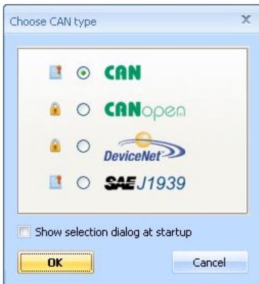
The bus system is selected by creating a new document using the menu "File" → „New..." of the CBT2 application software (Figure 7 refers).
